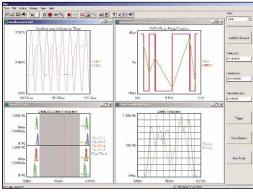
VISI software can provide multiple views of the same data (upper), or simultaneous views of several related data sets (lower), for at-a-glance analysis.
